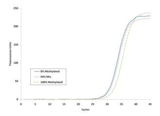
**Real-Time Amplification Plot.** This figure shows robust real-time amplification of 10 ng of bisulfite-converted human DNA using the  $\mathsf{Zymo}Taq^\mathsf{TM}$  qPCR PreMix and primers designed to amplify a region of the  $\mathit{MGMT}$  promoter.
